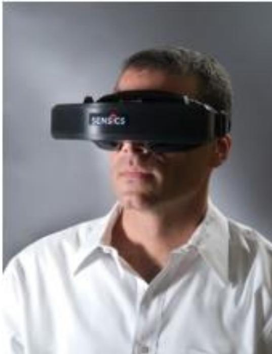
Figure 1. A closed-view head-mounted display. (Photo: [2])
