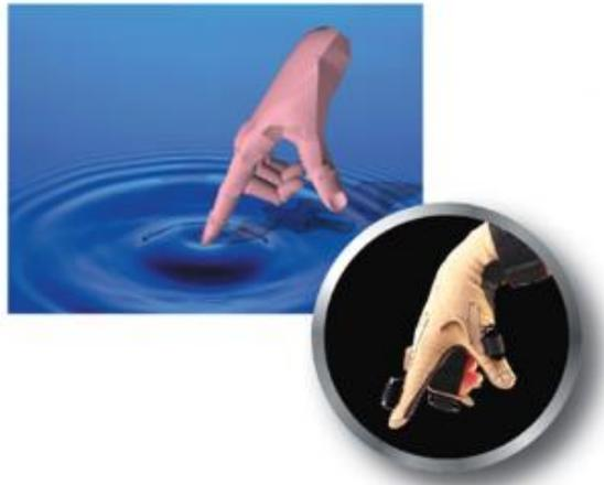
Figure 6. Tactile data glove SensAble's CyberTouch (Photo: [18])
